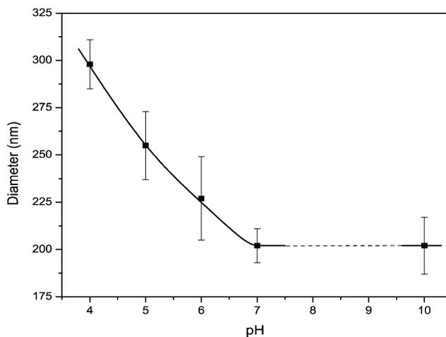
Fig. 5. Mean diameter of the particles as a function of pH.
