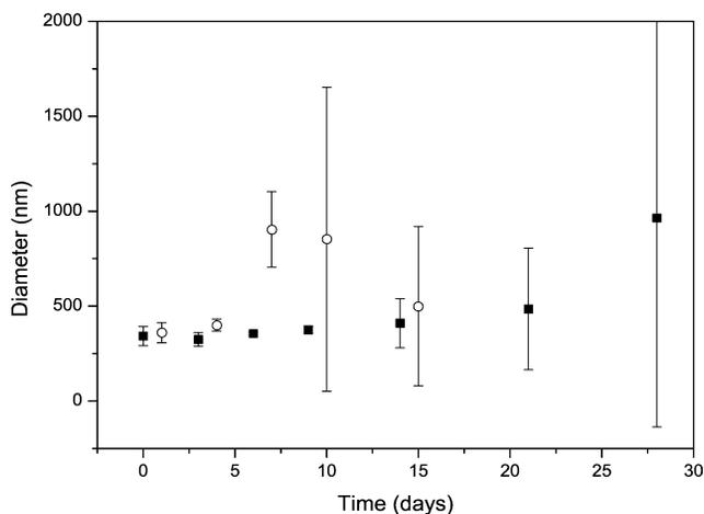
Fig. 1. Average diameter of chitosan nanoparticles stored at  $5^\circ\text{C}$  (■) and  $22^\circ\text{C}$  (○) as a function of time. Incubated in a nonbuffered solution (pH in the range 5–6) containing 1 mM of KBr.
