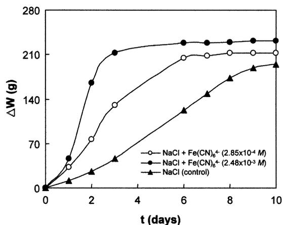
Fig. 3. Weight loss (due to evaporation) of the saline solution flowing through the porous stone) vs. time for the solutions without (control) and with additive.
