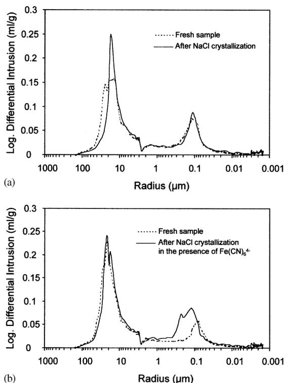
Fig. 5. Mercury intrusion porosimetry plots showing pore size distribution (i.e.,  $\log(dv/dr)$  vs.  $r$ , where  $v$  is the intruded volume and  $r$  the pore radius), for a control sample (a) and a sample submitted to NaCl crystallization in the presence of  $2.6 \times 10^{-3}$  M  $[\text{Fe}(\text{CN})_6]^{4-}$  (b). In both cases it is shown the curve corresponding to the stone before any crystallization occurred (dotted line) and after crystallization (solid line).
