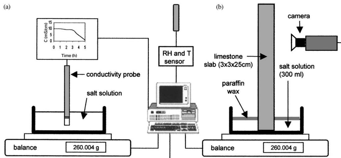
Fig. 1. Experimental set-up for sodium chloride crystallization: (a) open beakers, and (b) crystallization within porous stones (flow-through tests).
